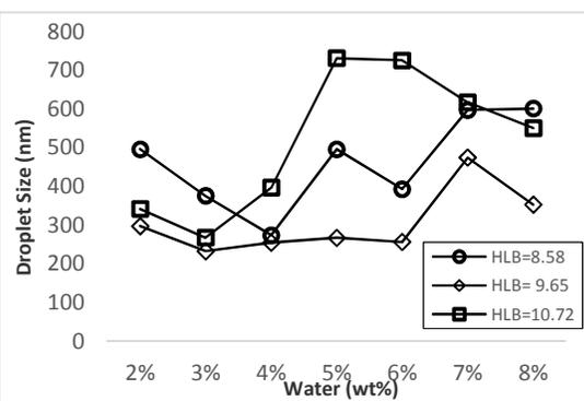
**Fig 3.** Droplet size of nano-emulsions as a function of water percentage (wt%). Surfactant HLB of the samples were fixed at 8.58, 9.65 and 10.72 respectively
