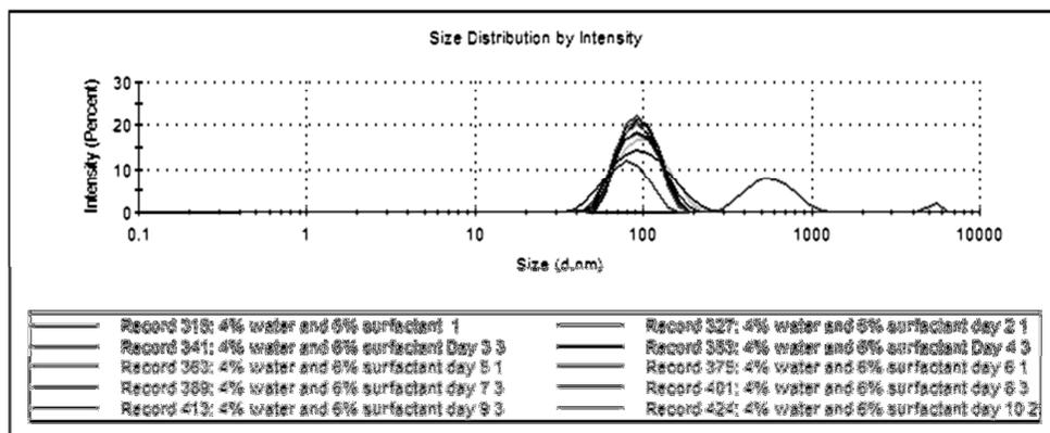
**Fig 9.** Dynamic Light Scattering (DLS) measurement for water-in-diesel nanoemulsion with 4 wt% water, throughout 10 days of storage
