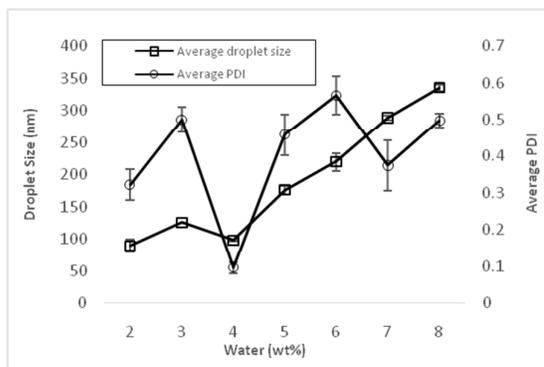
**Fig 2.** Droplet size of nano-emulsions as a function of water percentage (wt%). Surfactant wt% was fixed at 6 wt%
