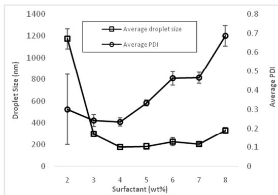
**Fig 1.** Droplet size and PDI of water-in-diesel nano-emulsions as a function of surfactant weight percentage (wt%)
