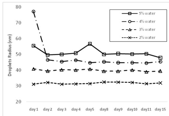
Fig 10. Stability of nano-emulsion with varying water content ( $S_{20}/T_{80}=6/4$ ,  $HLB = 11.16$ ).
