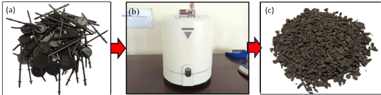
Fig.2. Material preparation (a) Resin waste (RW) from IC packages electronic industry; (b) Grinder Machine Fritsch's Planetary Mono Mill Pulverisette 6 Classic Line (c) Grinded resin waste
