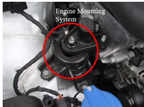
Fig. 1. Engine mount (samarins.com)
