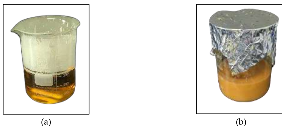
Fig. 1. TiO 2 Color Transformation a) Leaves extract mixed with TTIP solution b) Leaves extract mixed with TTIP solution after 8 hours stirred
