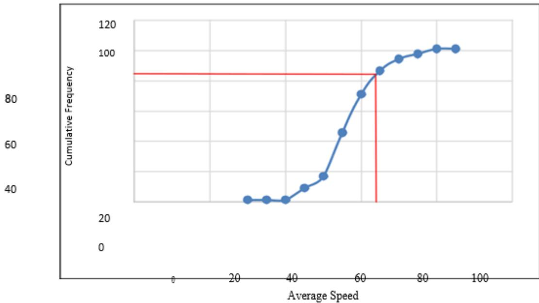
**Fig.11.** The graph of cumulative frequency against average speed at mid-curve during night time with a posted white speed limit signage
