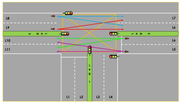
Fig.3. Observing Motorcycle Path for Straight Path at Three-legged Signalised Junction
