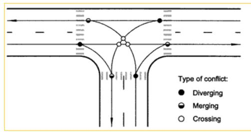
Fig.1. Traffic Conflict at three-legged Signalised Junction
