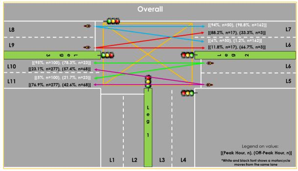
Fig.7. Motorcycle Path for Straight Movement
