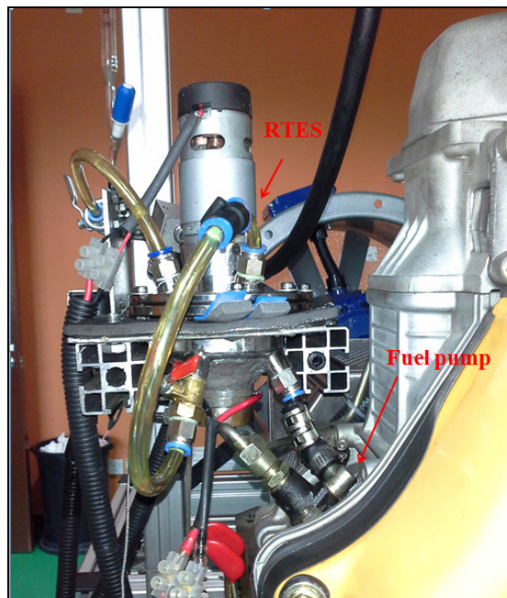
Figure 3: Location of RTES during the engine test
