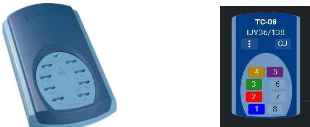
Fig. 3. PicoLog TC-08 used to log real-time temperature data from thermocouple
