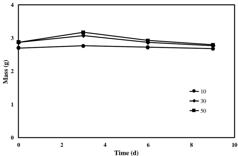
**Figure 3.** Mass Changes of Bio-composite during Accelerated Aging Test
