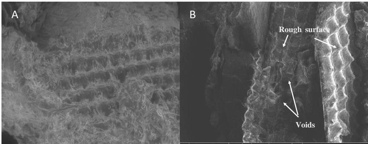
**Figure 2.** The view of 30 % rice husk, 70 % PLA at 500× under SEM (A) before tensile test, (B) after tensile test.
