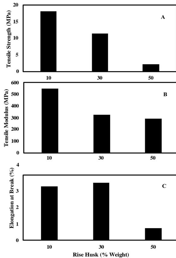
**Figure 1.** Tensile test of rise husk/PLA biocomposite (A) Tensile strength, (B) Tensile modules, (C) Elongation at break.
