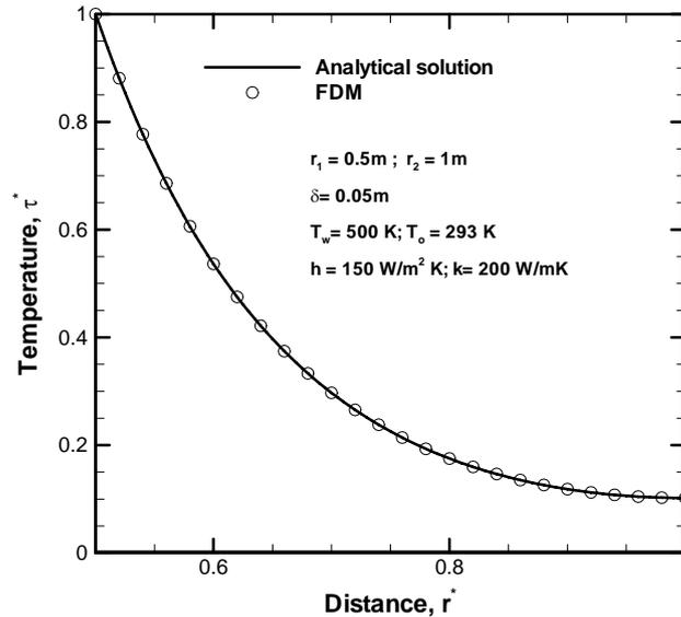
Figure 2: Validation of the forward model (FDM) with analytical solution
