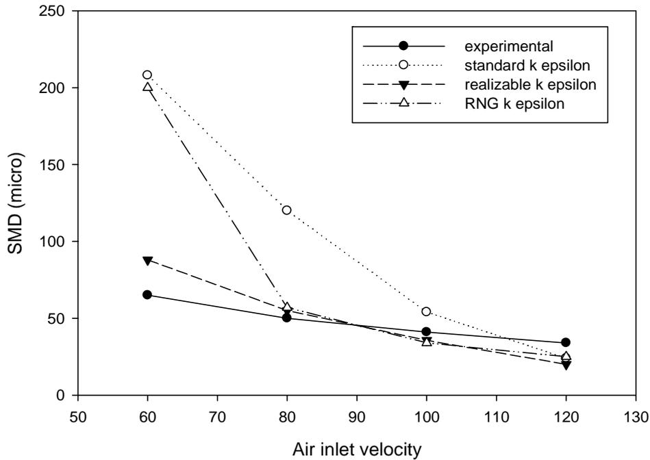
Figure 1. Comparison of three turbulence models with experimental data at four different air inlet velocities
