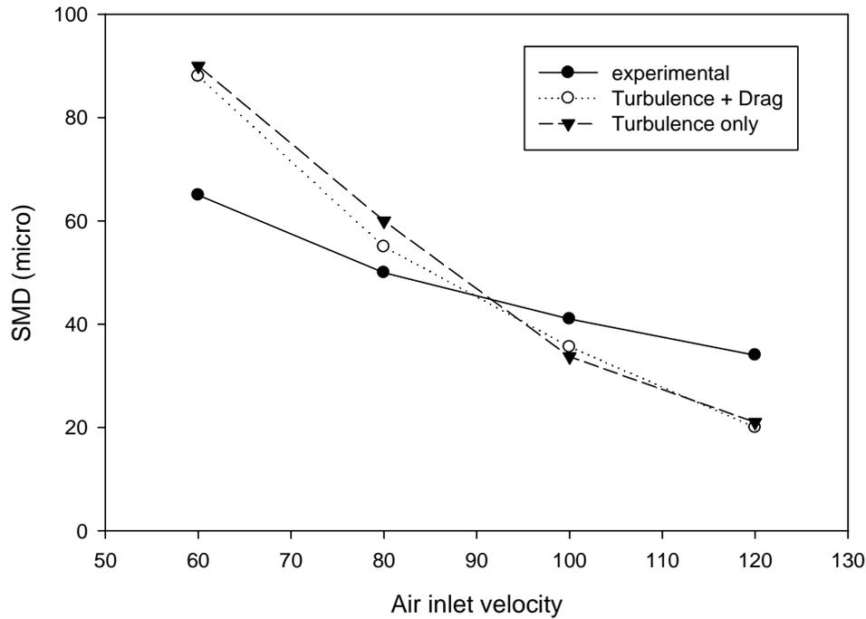
Figure 4 Comparison between the pure turbulence code and the combined turbulence and drag code with experimental data
