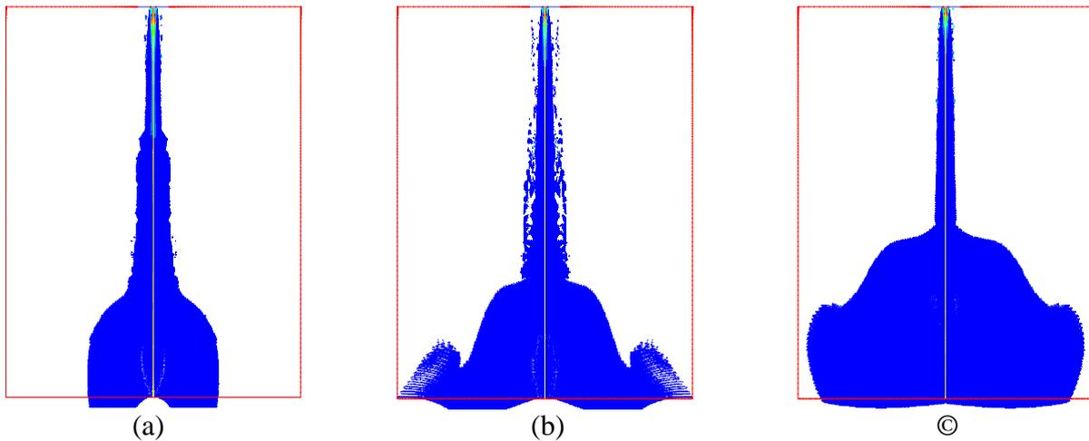
Figure 2. Spray patterns at different air inlet velocities (a)  $v=80$  m/s, (b)  $v=100$  m/s, and (c)  $v=120$  m/s
