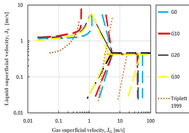
**Fig. 8.** Comparison between present result flow pattern maps and Triplett *et al.*, (1999)
