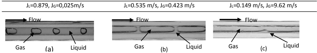
**Fig. 2.** A typical two-phase flow pattern based on  $J_L$  and  $J_G$  variations, (a) Bubble, (b). Plug, (c). Slug annular/Annular
