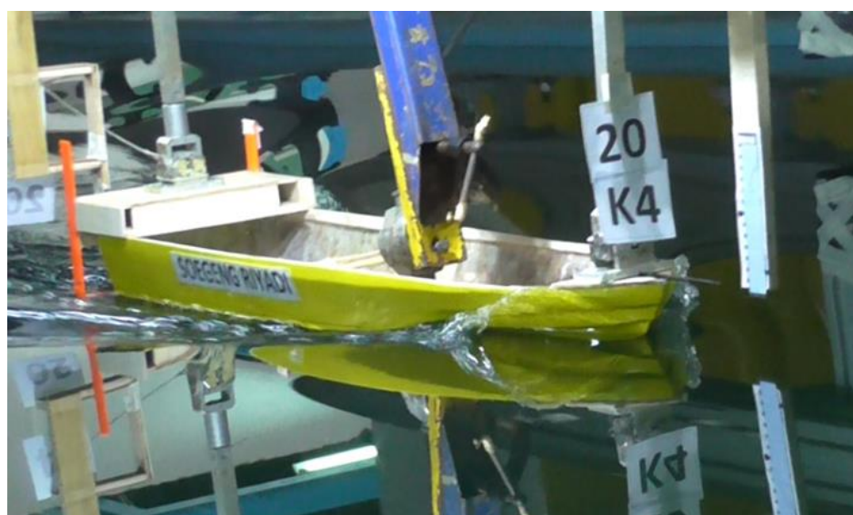
Fig. 5. Ship model towed at a speed of 1.62 m/s ( Fr = 0.62 ) for Case 3. The locally high water-overflow near the bow is partly ascribed to the hard chine body
