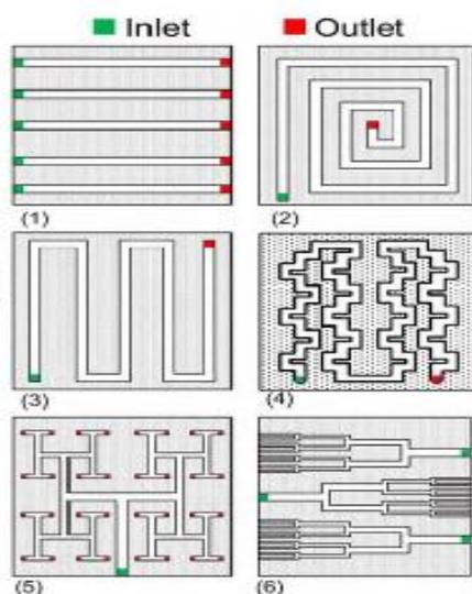
**Fig. 1.** Type of microchannel network
