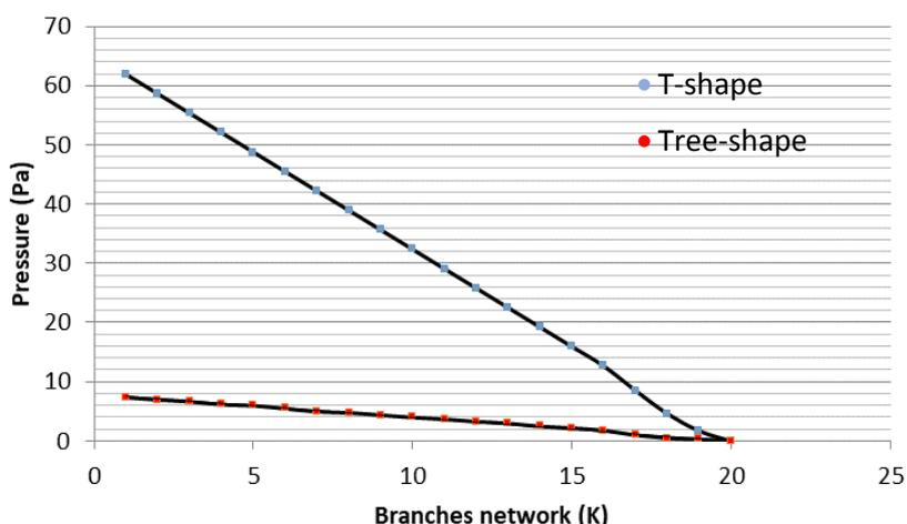
**Fig. 8.** Frictional pressure drop and pressure drop across a bifurcation at different branching level
