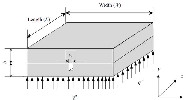
**Fig. 2.** Schematic of microchannel heat sink
