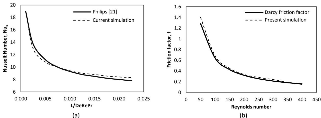
**Fig. 5.** Simulation model validation (a) Nusselt number (b) Friction factor
