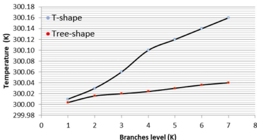
**Fig. 7.** Temperature distribution at constant heat flux,  $q=325 \text{ W/cm}^2$  for Tree-shaped and T-shaped fractal
