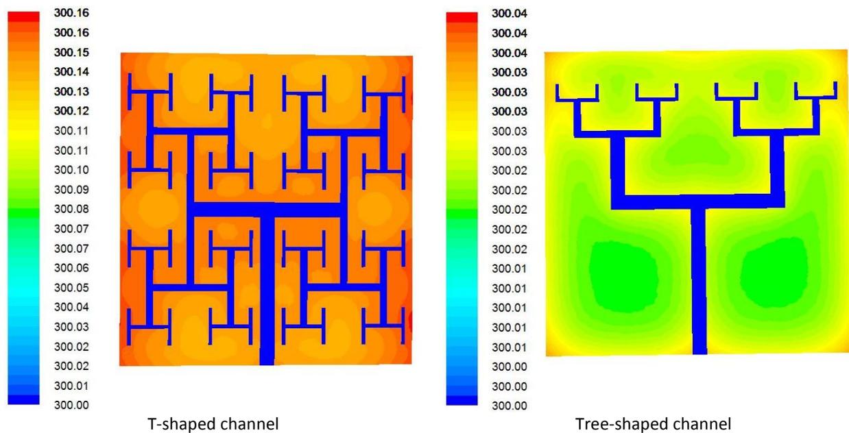
**Fig. 6.** Temperature distribution at the bottom of heat sink
