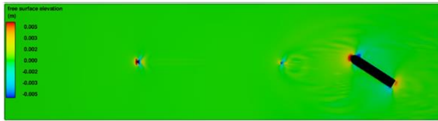
Fig. 9. Free surface elevation, V_s = (a) 0.509, (b) 0.582, and (c) 0.653 m/s
