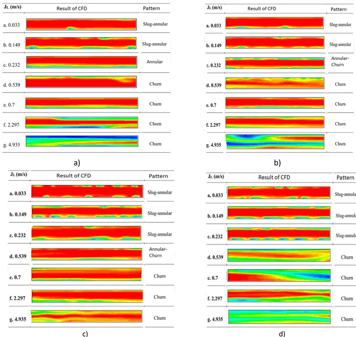
**Fig. 1.** The Flow Pattern with  $J_G = 9.62$  m/s and Various Variation of  $J_L$  a) Air-Water with 0% Glycerine, b) Air-Water with 10% Glycerine, c) Air-Water with 20% Glycerine, and d) Air-Water with 30% Glycerine
