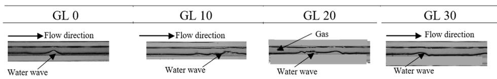
**Fig. 4.** Experimental data of Flow Pattern with  $J_G = 4.238 \text{ m/s}$  and  $J_L = 0.091 \text{ m/s}$  with various concentration of glycerin
