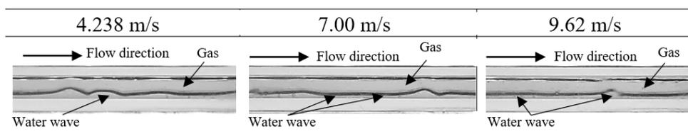
**Fig. 3.** Experimental data of Flow Pattern with  $J_L = 0.149$  m/s and Various of  $J_G$  with concentration of 20% glycerine
