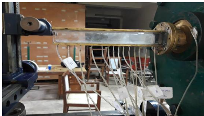
Fig. 1. A view of the nozzle along with the duct attached with the settling chamber of the open jet facility
