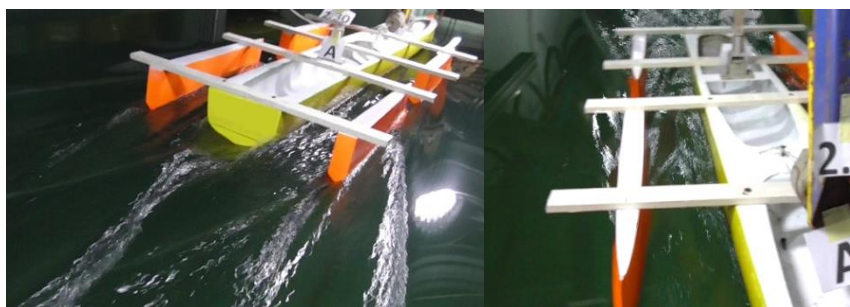
Fig. 11. Wave characteristic of test results of models A, C and E at Fn 0.6 between the main hull and the side hull (right), and after stern (left)
