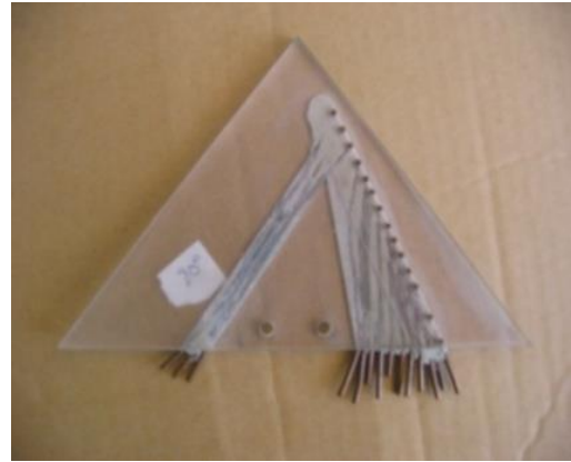
Fig. 1. Pressure taps positions under apex vortex of a delta wing model. Right: Model schematic view and left: realized model
