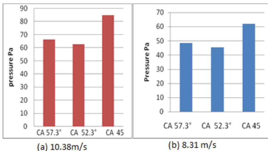
**Fig. 13.** Influence of cone angle (CA) on pressure drop corresponding to inlet velocity 10.38m/s and 8.31 m/s
