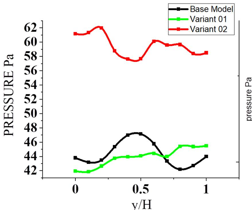
**Fig. 9.** Pressure Vs. the non-dimensional distance along with the diagonal path correlative to 10.38 m/s inlet velocity at  $v_1$  location
