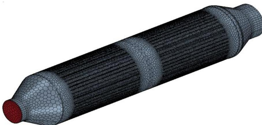
Fig.2. The meshed fluid domain of catalytic converter
