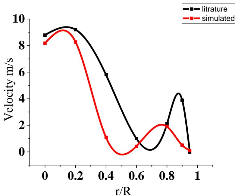
**Fig. 4.** Momentum intensity Vs. non-dimensional diagonal coordinate at location  $v_1$
