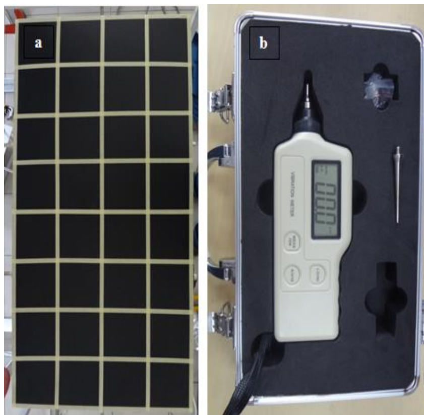
Fig. 5. Photograph of a: PV with 45 points upper surface division, b: Portable vibration meter
