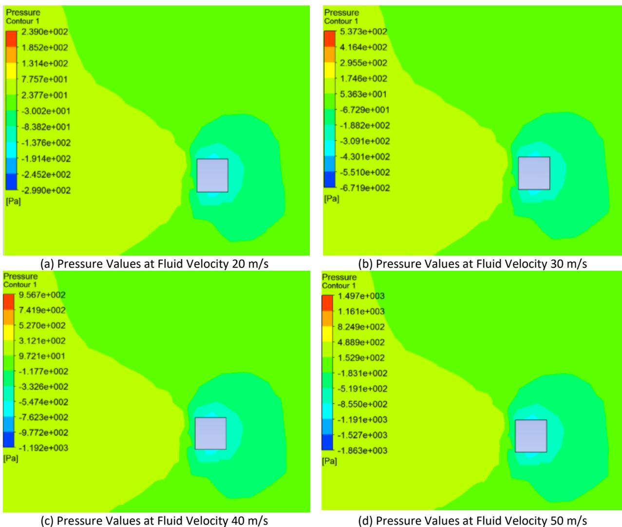
**Fig. 4.** Pressure contours of fluid striking rooftop at 0°
