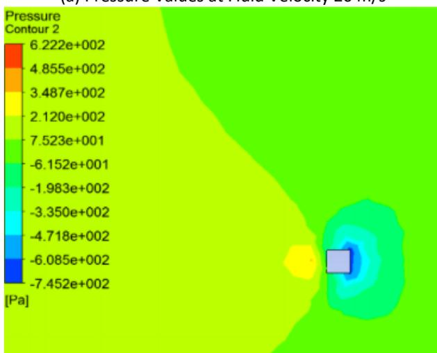
(c) Pressure Values at Fluid Velocity 40 m/s
