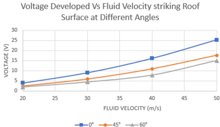
Fig. 7. Voltage vs fluid velocity comparison
