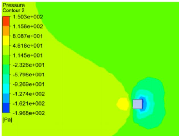
(a) Pressure Values at Fluid Velocity 20 m/s
