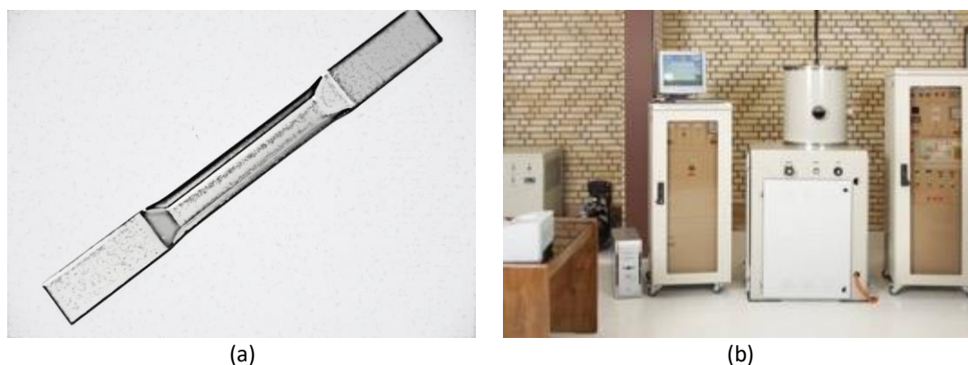
Fig. 4. (a) Tungsten boat (b) The thermal evaporation unit
