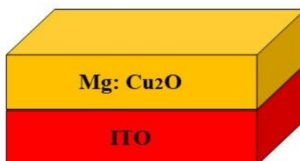
Fig. 1. Illustration cell configuration of Mg doped Cu 2 O on ITO substrate glass
