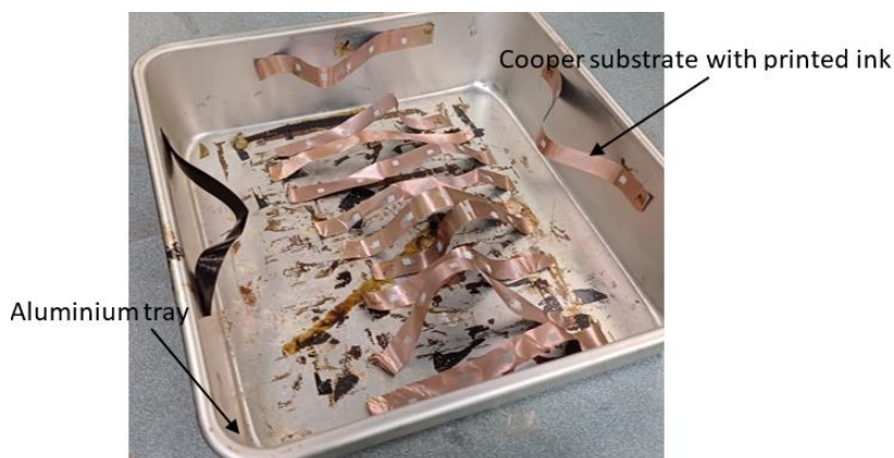
Fig. 18. GNP/Ag conductive ink for curing process
