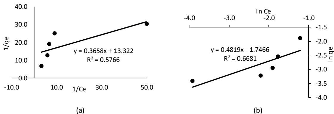
**Fig. 9.** Linear plot of (a) Langmuir model of  $1/q_e$  against  $1/C_e$  for the adsorption of  $PO_4^{3-}$  onto adsorbent from domestic wastewater (b) Freundlich model of  $\ln(C_e)$  against  $\ln(q_e)$  for the adsorption of  $PO_4^{3-}$  onto adsorbent from domestic wastewater
