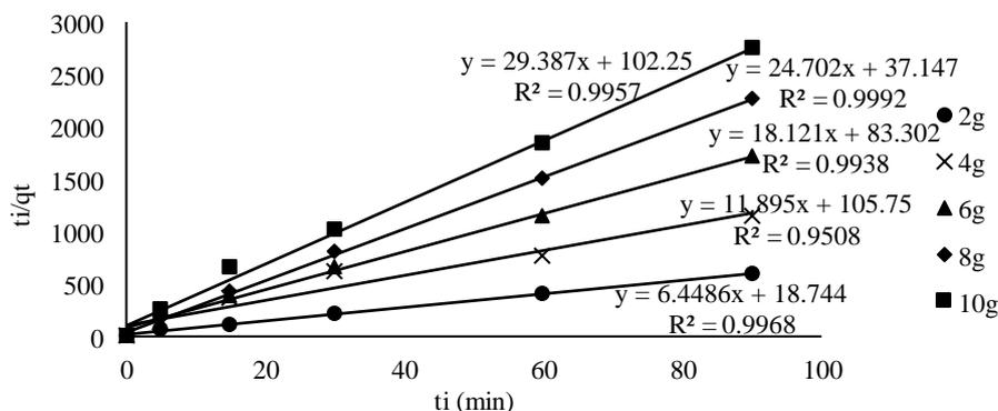
**Fig. 8.** Pseudo-second-order analysis graph (Plot of linear regression model of pseudo-second-order for the adsorption of  $\text{PO}_4^{3-}$  onto adsorbent from domestic wastewater)
