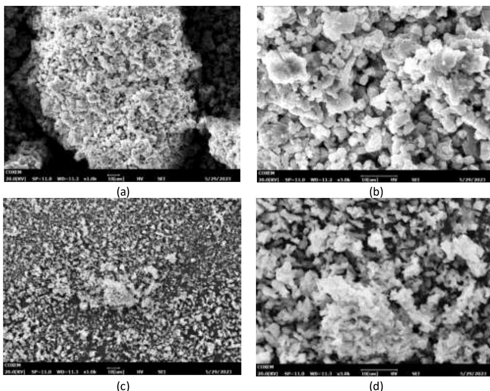
**Fig. 2.** Surface morphology of the adsorbent before: (a) at 1000× magnification (b) at 3000× magnification, after: (c) at 1000× magnification (d) at 3000× magnification
