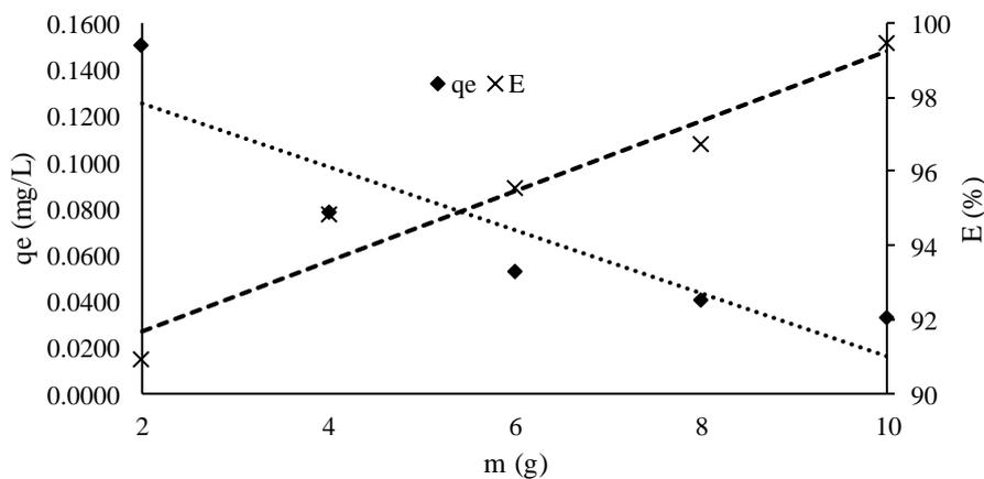
**Fig. 6.** Effect of the different masses of the adsorbent on the adsorption capacity,  $q_e$  and removal efficiency,  $E$  (%)
