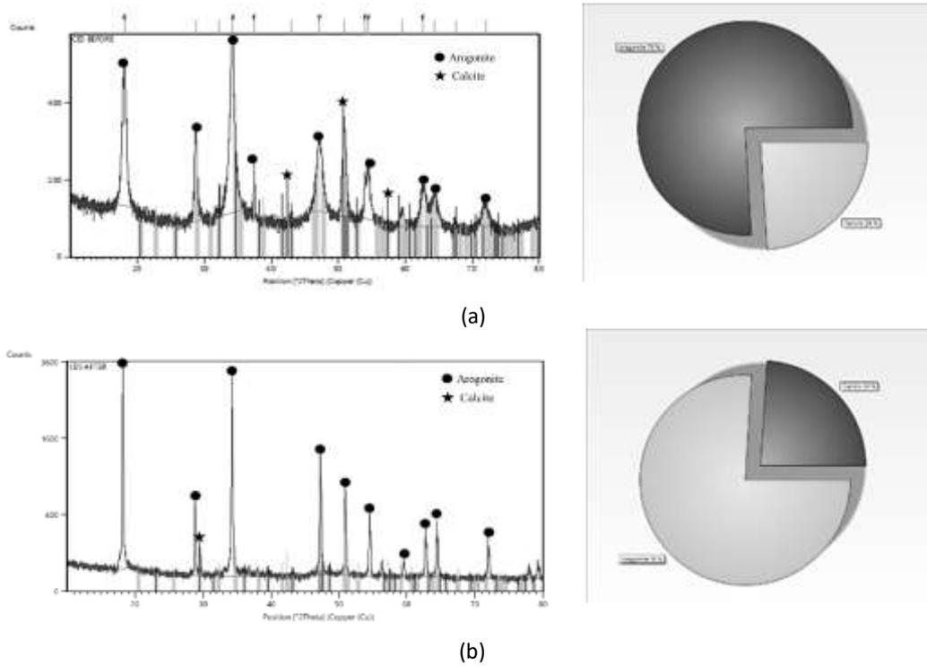
**Fig. 3.** XRD spectra of aragonite and calcite components of the adsorbent (a) before adsorption and (b) after adsorption
