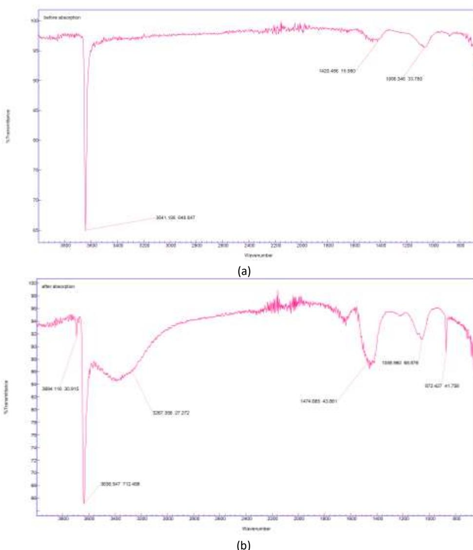
**Fig. 1.** FTIR spectra of adsorbent (a) before adsorption and (b) after adsorption of phosphorus ( $\text{PO}_4^{3-}$ )
