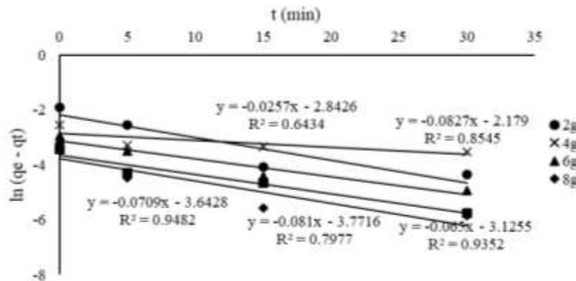
**Fig. 7.** Pseudo-first-order analysis (Plot of linear regression model of pseudo-first-order for the adsorption of  $\text{PO}_4^{3-}$  onto adsorbent from domestic wastewater)
