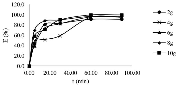
**Fig. 5.** The performance of removal efficiency,  $E$  (%), against time,  $t$  (min), for every particle mass
