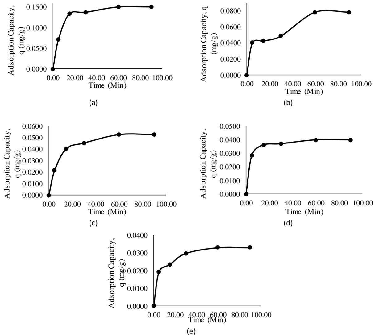
**Fig. 4.** Effect of adsorption capacity on phosphorus removal for (a) 2 g (b) 4 g (c) 6 g (d) 8 g and (e) 10 g
