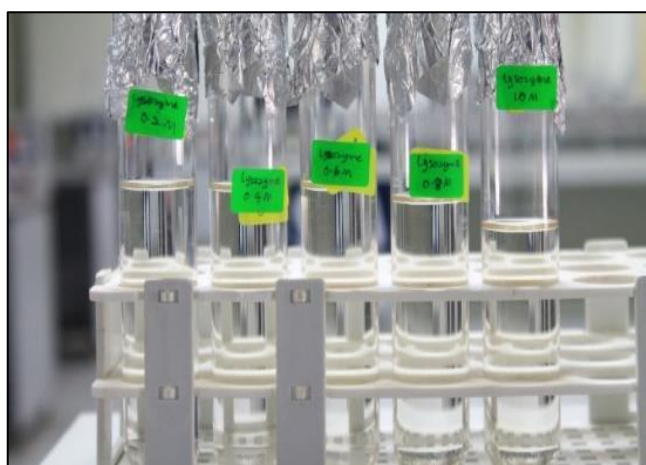
Fig. 1. Lysozyme at different molarities was placed in the test tube and diluted with 50 ml distilled water
