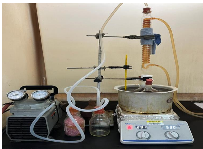
Fig. 1. Set-up of the transesterification process
