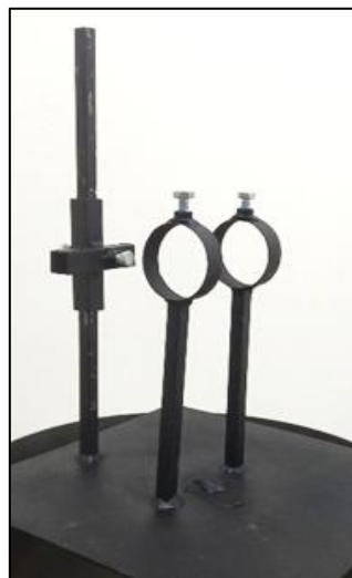
Fig. 6. AerospaAcer stand used to hold AerospaAcer inside wind tunnel
