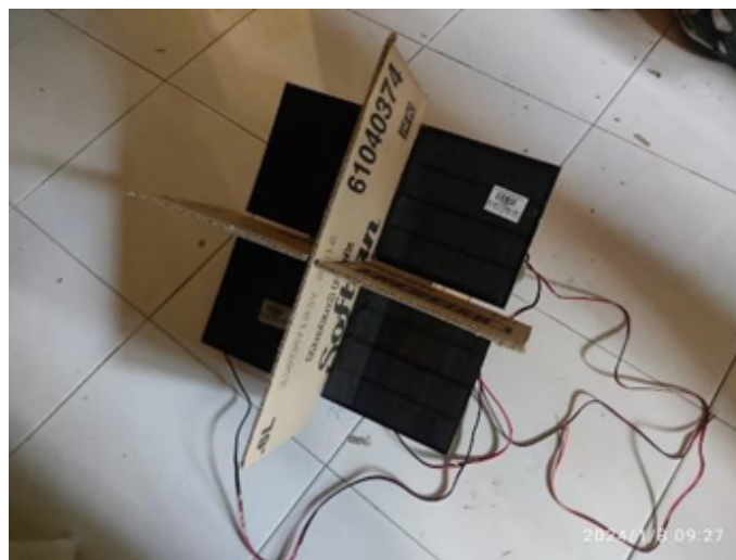
Fig. 4. Low-cost solar tracker using shadow detection experimental setup
