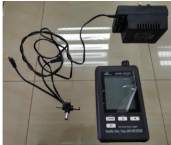
Fig. 2. Air temperature measure device, Humidity + thermometer + barometer LUTRON MHB-382SD
