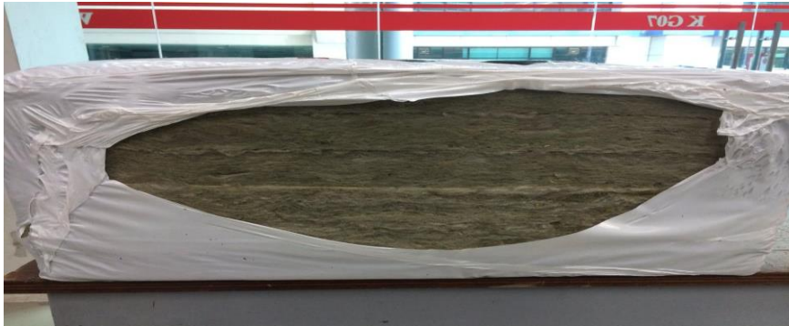
Fig. 1. Rockwool pack containing 6 layers, each of 50mm thickness
