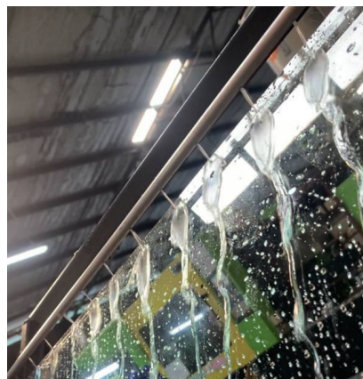
Fig. 2. The water flows out from the bladeless wiper rod
