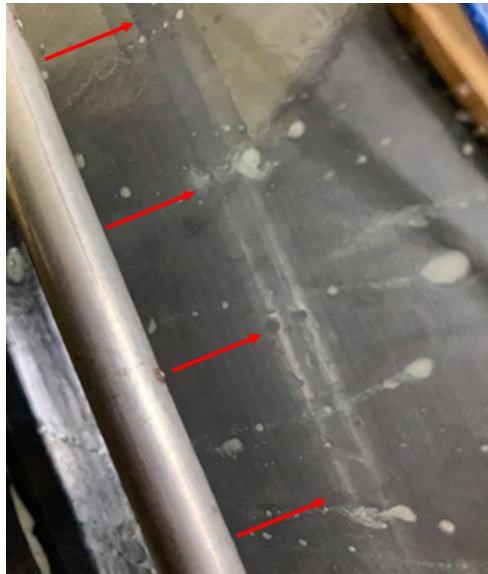
Fig. 3. The air flows out of the 1mm hole in the wiper rod
