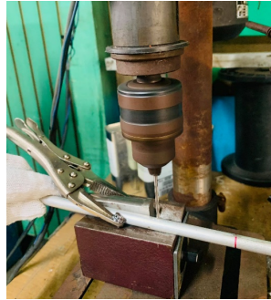
Fig. 18. Hollow aluminium rods milling process
