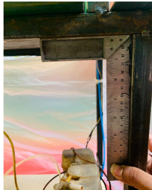
Fig. 12. Using a 'L' shape ruler for right angle measurement
