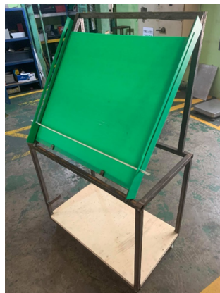
Fig. 13. Fabrication of the smart wiper washing system frame
