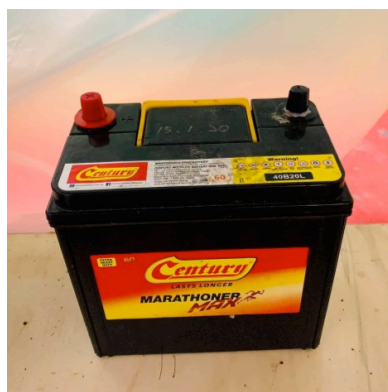
Fig. 30. 12v battery, model: 35Amps, CCA- 342Amps, 6 plates, 35Ah standard din
