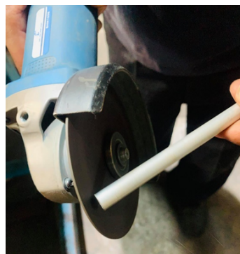
Fig. 16. Process of smoothing the hollow aluminium rod
