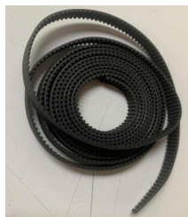
Fig. 24. Actual image showing gear belt of type GT2 6mm timing belt used for the current work
