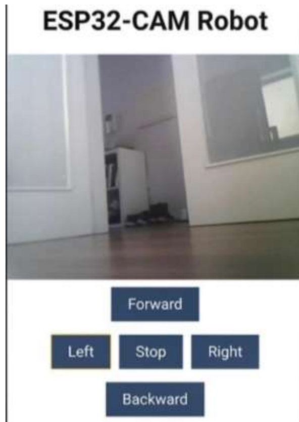
Fig. 9. Virtual joystick and online video streaming
