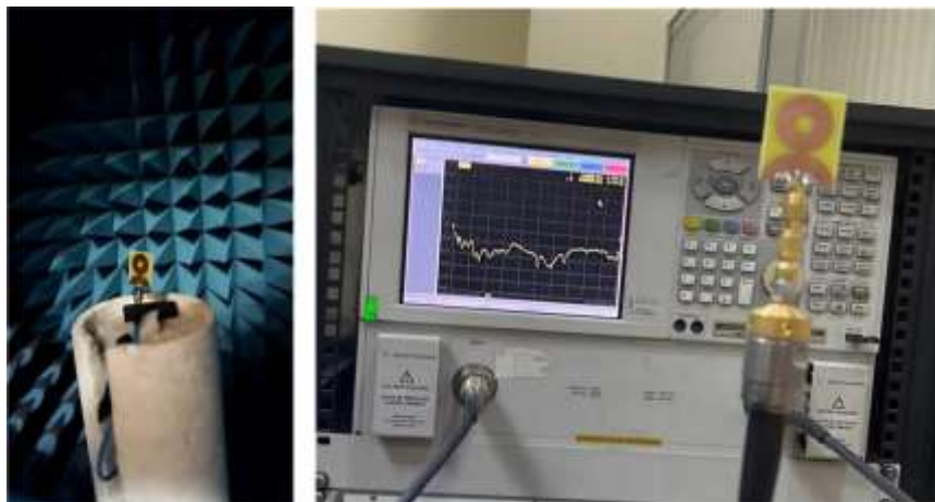
Fig. 9. The measurements set (a) the proposed antenna in the anechoic chamber and (b) S11 measurements
