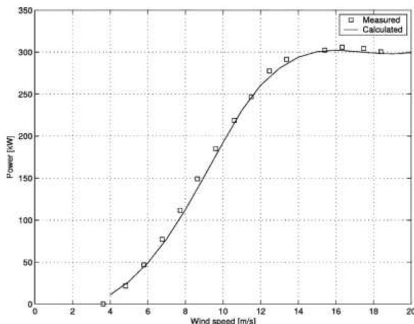
Fig. 2. Power curve of the Bonus 300 kW wind turbine [40]
