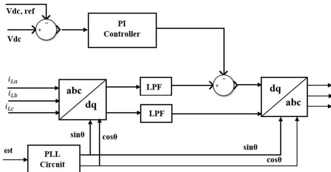
Fig. 3. Block diagram for synchronous reference frame method
