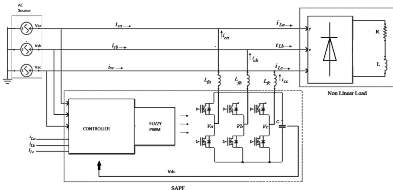
**Fig. 1.** Three phase shunt active power filter (SAPF) block diagram
