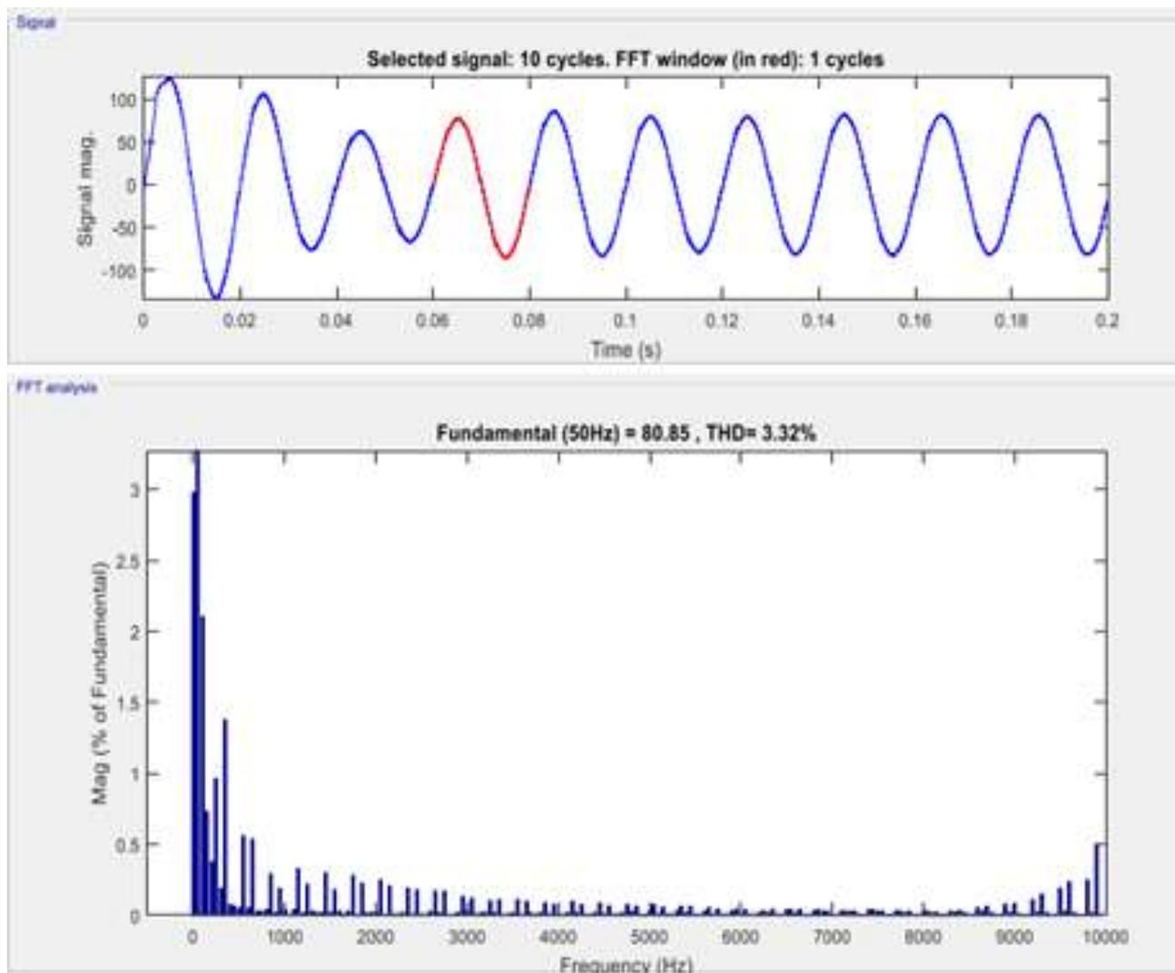
**Fig. 13.** Harmonic percent for DQ theory using PI and SPWM
