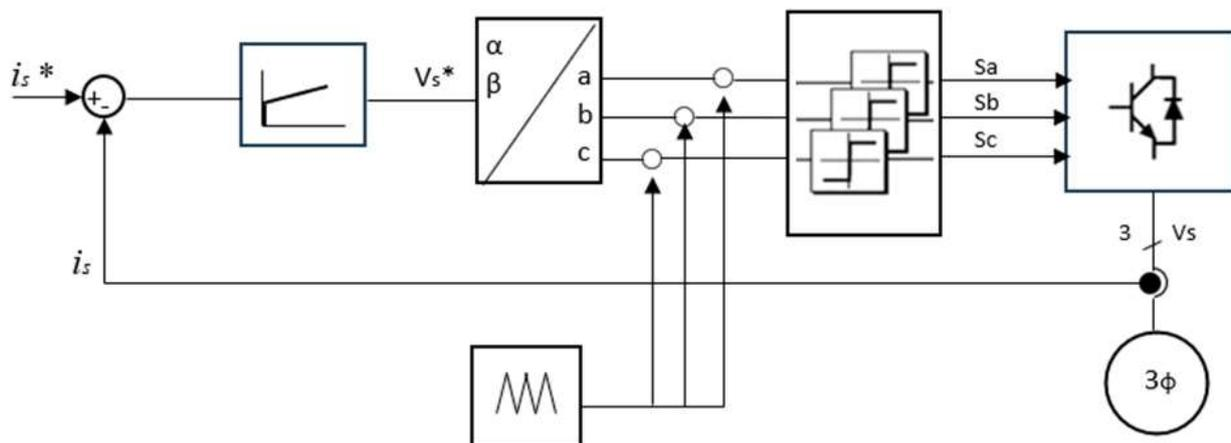
**Fig. 4.** Block diagram for SPWM current control scheme
