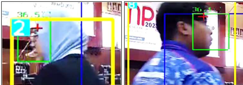
Fig. 7. The body temperatures of two individuals have been recorded. Both individuals exhibit normal body temperatures, as indicated by the presence of green bounding boxes around them
