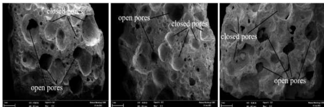
Fig. 6. Open pores and closed pores of AAC-GIW
