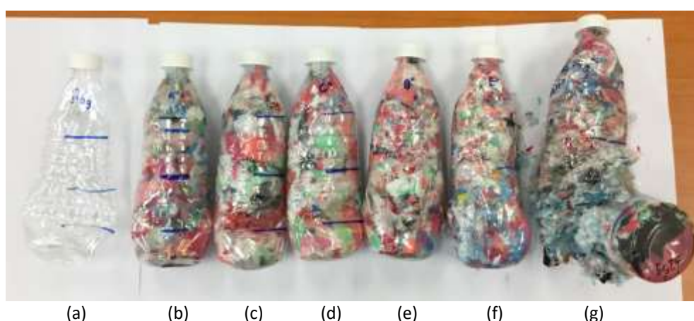
Fig. 6. Ecobrick sample after the flexural test (a) Sample A (b) Sample B (c) Sample C (d) Sample D (e) Sample E (f) Sample F (g) Sample G
