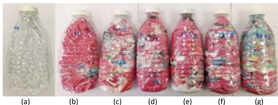
Fig. 3. Ecobrick sample after compressive test (a) Sample A (b) Sample B (c) Sample C (d) Sample D (e) Sample E (f) Sample F (g) Sample G
