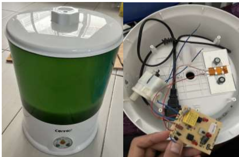
Fig. 1. Original body and electric circuit of current machine
