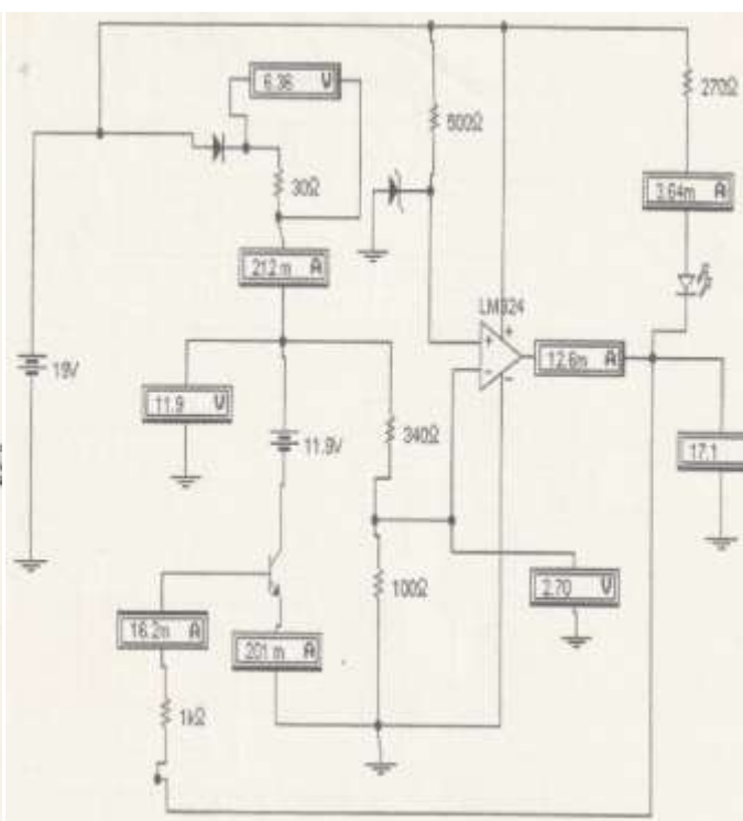
Fig. 3. 12V battery charging circuit diagram
