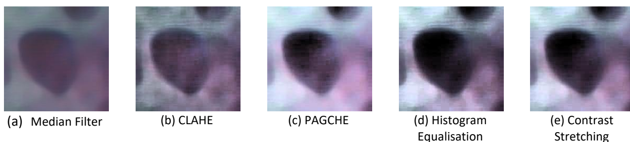
Fig. 16. Experimental results of Image 3 after applying Median Filter followed by contrast enhancement methods (b-e)
