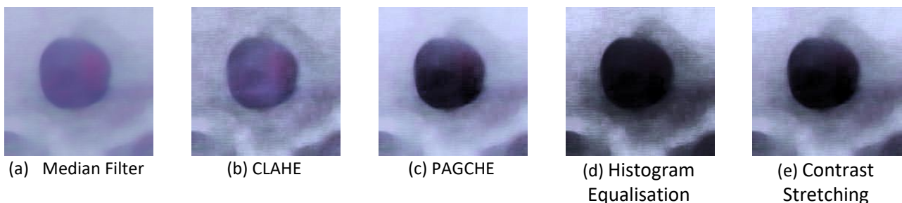
Fig. 8. Experimental results of Image 1 after applying Median Filter followed by contrast enhancement methods (b-e)
