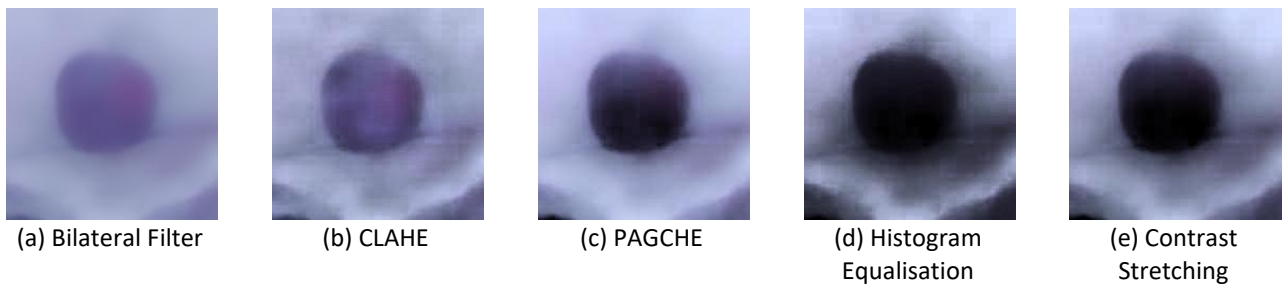
Fig. 7. Experimental results of Image 1 after applying Bilateral Filter followed by contrast enhancement methods (b-e)
