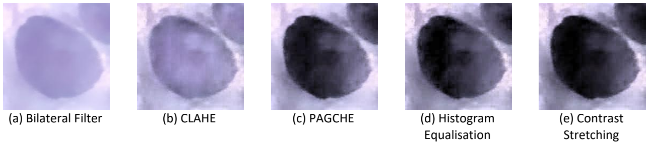
Fig. 19. Experimental results of Image 4 after applying Bilateral Filter followed by contrast enhancement methods (b-e)
