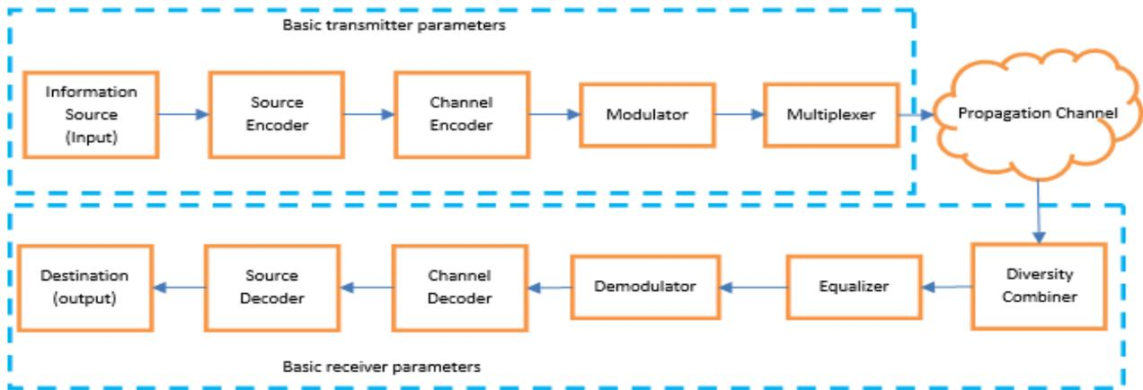
**Fig. 1.** Block diagram of wireless communication
