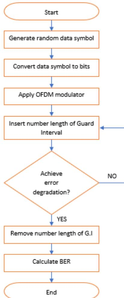
**Fig. 2.** Flow chart of GI deployment in the system
