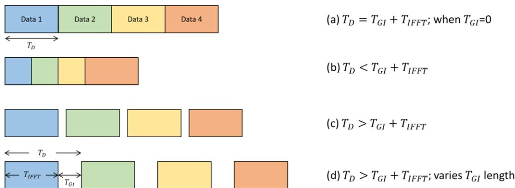
**Fig. 4.** OFDM frame with GI extension
