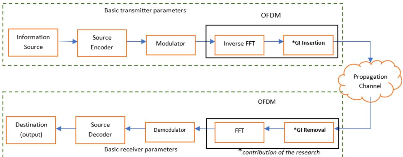
**Fig. 3.** GI inserted in OFDM System
