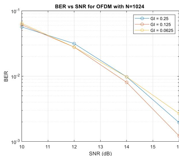
**Fig. 7.** Simulated with  $N_{fft}$  1024
