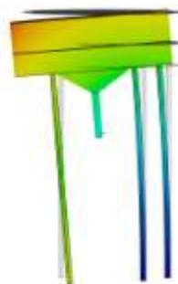
**Fig. 9.** Displacement results of the filtration tank
