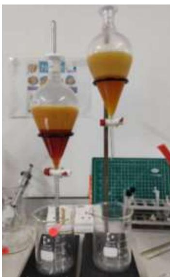
**Fig. 4.** Washing process to remove the impurities in FAME
