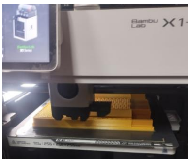
Fig. 4. 3D printing process by Bambu Lab X1 carbon printer
