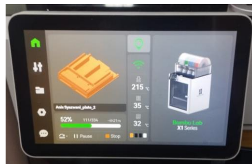
Fig. 4. 3D printing process by Bambu Lab X1 carbon printer
