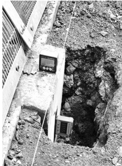
Fig. 3. Inclinometer for record deflection of foundation
