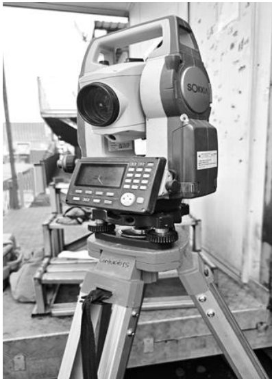
Fig. 2. Total station for record deflection of fence line post
