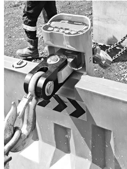
Fig. 4. Electronic crane scale with capacity 10 Ton
