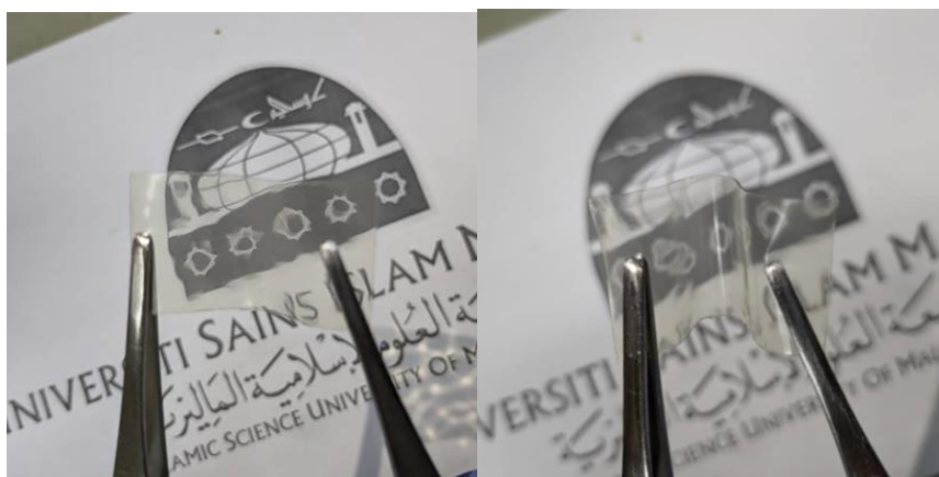
Fig. 2. A clear, free-standing, flexible 2-HEC based SBE
