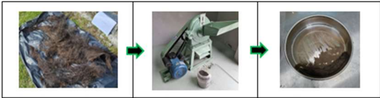
Fig. 2. Process to have fine SPF (a) Raw sugar palm fiber (b) Crushed process (c) Sieve process
